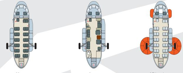
26-seat passenger layout 9-seat VIP passenger layout Offshore layout
